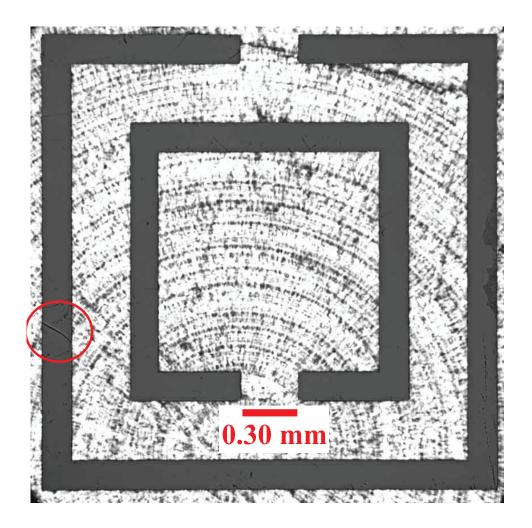
Figure 5.14: An optical image of the single Nb split-ring resonator $-\beta$ . Note surface defects on the Nb film. The rings in the background were from the cold-finger that the single Nb split-ring resonator $-\beta$  was placed upon. A scratch on the left side on the outer ring is circled in red.
