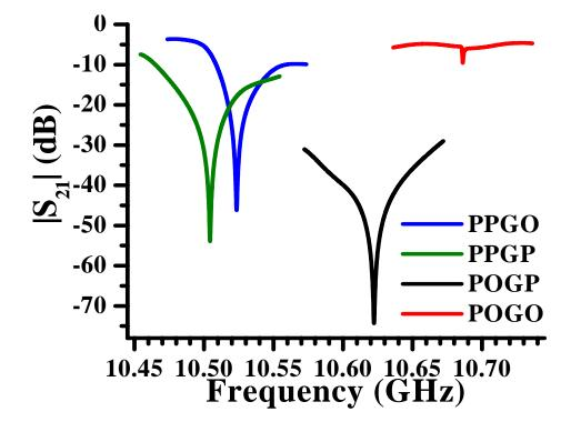
Figure 5.21: A plot of the electromagnetic transmission,  $|S_{21}|$ , versus frequency for the single Nb split-ring resonator— $\pi$ , inside the Nb X-band waveguide immersed in liquid Helium. The curves are labeled as follows: PPGO (blue): plane-parallel gap-orthogonal; PPGP (green): plane-parallel gap-parallel; POGP (black): plane-orthogonal gap-parallel; POGO (red): plane-orthogonal gap-orthogonal. The orientations were described in Figure (2.10).
