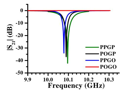
Figure 5.22: A plot of the electromagnetic transmission,  $|S_{21}|$ , versus frequency for a simulation of a single split-ring resonator made of a perfect electric conductor. The curves are labeled as follows: PPGO (blue): plane-parallel gap-orthogonal; PPGP (green): plane-parallel gap-parallel; POGP (black): plane-orthogonal gap-parallel; POGO (red): plane-orthogonal gap-orthogonal. The orientations were described in Figure (2.10).
