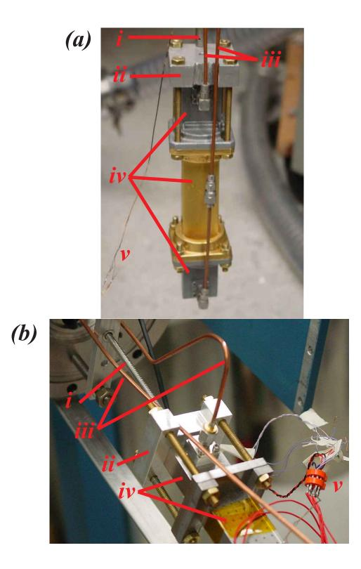
Figure 3.11: The experimental probes. (a) Small Dewar probe. (b) Large Dewar probe. Both figures contain numbers that refer to the same features: (i) support rod; (ii) Al block; (iii) coaxial cables; (iv) waveguide and couplers; (v) thermometer (and heater for (b)).
