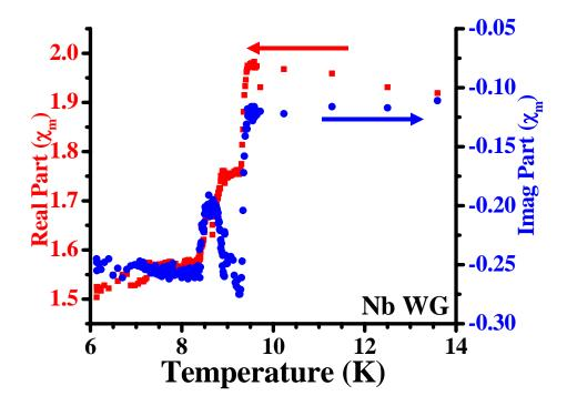
Figure 3.6: The ac magnetic susceptibility, ,  $\chi_m$ , versus temperature, of the Nb X-band waveguide, labeled Nb WG. The red squares denote the real part of the ac magnetic susceptibility, while the blue circles denote the imaginary part of the ac magnetic susceptibility.
