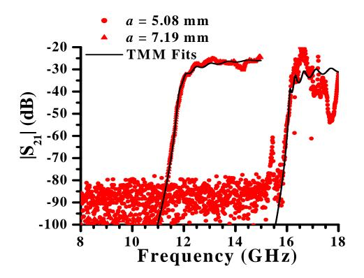
Figure 4.7: A plot of the electromagnetic transmission,  $|S_{21}|$ , versus frequency for a Nb wire array in the Ag-plated brass X-band waveguide at room temperature. The red circles are the data for the lattice parameter of a = 5.08 mm, while the red triangles are the data for the lattice parameter of a = 7.19 mm. The black curves are the fits from the three-layer transfer matrix model.
