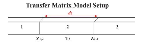
Figure 2.7: Setup of the three-layer transfer matrix model inside a waveguide. The layers are labeled 1, 2, 3, with the associated impedance matrix,  $Z_{ij}$ , and transmission matrix,  $T_k$ , where i, j, k refer to a specific layer. Layers 1 and 3 extend to infinity, while layer 2 has thickness  $d_2$ .
