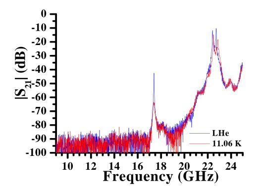
Figure 6.13: A plot of the electromagnetic transmission,  $|S_{21}|$ , versus frequency for a single Nb split-ring resonator in the *Ka*-band waveguide, measured in liquid Helium, shown as the blue curve, and 11.06 K, shown as the red curve.
