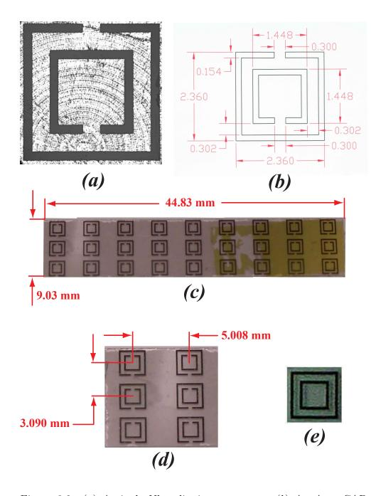
Figure 3.2: (a) A single Nb split-ring resonator. (b) An Auto-CAD drawing of a single split-ring resonator with dimensions, all in mm. (c) A split-ring resonator "chip," containing an array of three-by-nine Nb split-ring resonators. The yellow tape on the back right of the chip was used to connect two chips lengthwise in order to create a longer split-ring resonator array. (d) A close-up of the chip, with dimensions. (e) A Nb closed-ring resonator with the same dimensions as (b).
