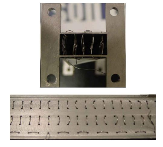
Figure 3.9: A Nb wire array in the Nb X-band waveguide, with a lattice parameter of a = 4.57 mm. The short lattice parameter prevented the wires from being pulled straight, and forced the wires inside the Nb Xband waveguide to be curved, as shown in the top of the figure. The bottom of the figure shows a view of the broadside of the Nb X-band waveguide from the outside.
