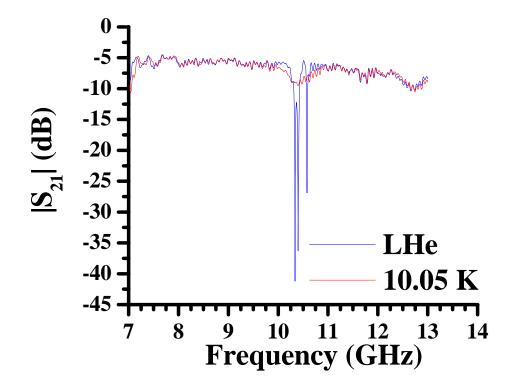
Figure 5.6: A plot of the electromagnetic transmission,  $|S_{21}|$ , versus frequency for an array of 3 Nb split-ring resonators, inside the Ag-plated brass X-band waveguide. The blue curve is data taken while the Ag-plated brass X-band waveguide and Nb split-ring resonators were immersed in liquid Helium, denoted LHe, while the red curve is data that was taken at 10.05 K.
