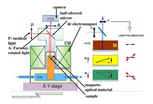
Figure 3.15: The experimental setup for the magneto-optical experiment. Incident light is directed to a sample with a half-silvered mirror. The sample is underneath a magneto-optical material, and an applied dc H field is orthogonal to the sample. The incident light experiences a Faraday rotation, shown in the right side of the figure. The Faraday rotated light travels to a charge-coupled device camera, and imaged.
