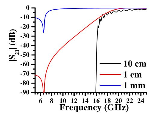
Figure 4.11: A plot of the electromagnetic transmission,  $|S_{21}|$ , calculated from the three-layer transfer matrix model with a plasmalike permittivity, versus frequency for various medium lengths. The black curve is a medium 10 cm in length, the red line a medium 1 cm in length, and the blue curve a medium 10 mm in length. The parameters used to calculate these curves were  $\omega_p = 2\pi \times 16$  GHz, and  $\gamma = 2\pi \times 100$  MHz.
