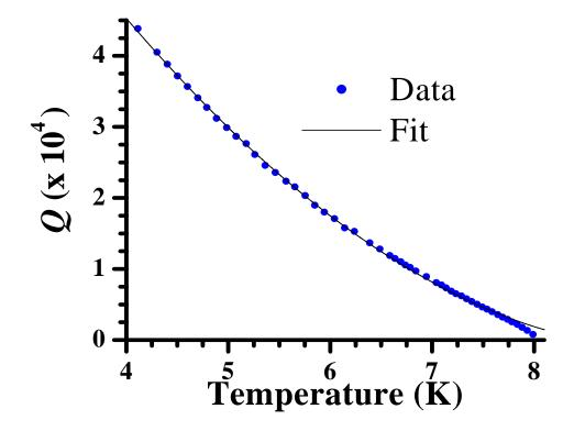
Figure 5.11: A plot of the quality factor, Q, versus temperature for the single Nb split-ring resonator- $\alpha$ . Note that this data is not taken from the data in Figure (5.9), but rather taken at a later time. The blue dots are the data, while the black curve is a fit using Equation (2.160).
