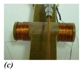
Figure 3.12: The superconducting solenoid used in the applied dc H field experiments, installed on the Ag-plated brass X-band waveguide. (a) The entire Ag-plated brass X-band waveguide with the solenoid. (b) and (c) Closeups of the solenoid on the Ag-plated brass X-band waveguide.
