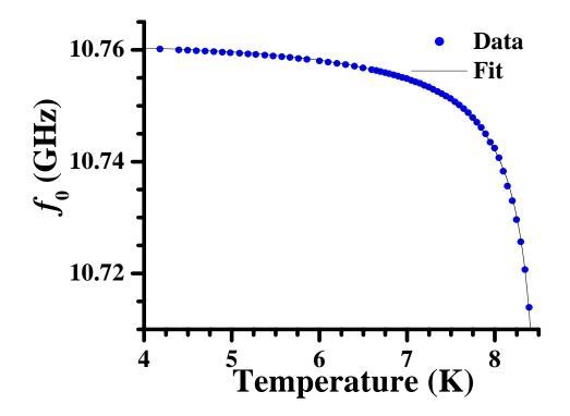
Figure 6.9: A plot of the resonant frequency,  $f_0$ , versus temperature for the single Nb split-ring resonator- $\alpha$  in a Nb wire array measuring five rows transversely and seven rows longitudinally, as in Figure (6.8). The blue dots are the data, while the black curve is a fit using Equation (2.151).
