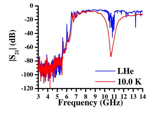
Figure 5.2: A plot of the electromagnetic transmission,  $|S_{21}|$ , versus frequency for an array of 216 Nb split-ring resonators, measured in liquid Helium, denoted by the blue curve, and at 10.00 K, denoted by the red curve, in the Ag-plated brass X-band waveguide. Rohacell® HF was used to orient the Cu-Ni-Au split-ring resonators.
