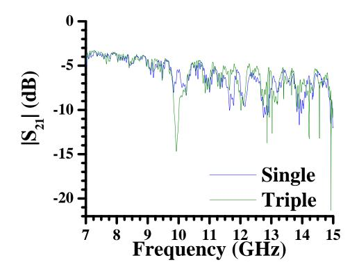
Figure 5.20: A plot of the electromagnetic transmission,  $|S_{21}|$ , versus frequency for an array of a single Cu-Ni-Au split-ring resonator, shown in blue, and three Cu-Ni-Au split-ring resonators, shown in green. The data were measured in the Ag-plated brass X-band waveguide with the Nb waveguide-to-coaxial cable couplers. The ringing in the data were due to standing waves in the coaxial cables, due to impedance mismatches in the entire circuit.
