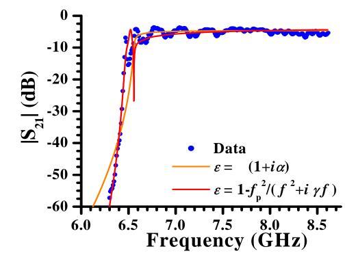
Figure 4.2: A plot of the electromagnetic transmission,  $|S_{21}|$ , versus frequency for an empty Ag-plated brass X-band waveguide immersed in liquid Helium, denoted by the blue circles, and two fits using the transfer matrix model. The red curve used a plasma-like permittivity, and the orange curve used a constant complex permittivity. Both used a relative permeability of  $\mu = 1$ .
