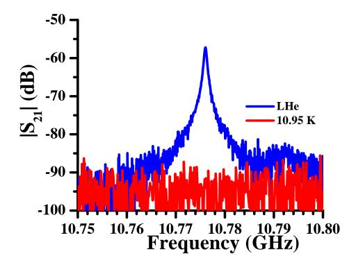
Figure 6.14: A plot of the electromagnetic transmission,  $|S_{21}|$ , versus frequency for the single Nb split-ring resonator- $\pi$  in the Ka-band waveguide-to-coaxial cable couplers, measured in liquid Helium, denoted LHe, shown as the blue curve, and 10.95 K, shown as the red curve.
