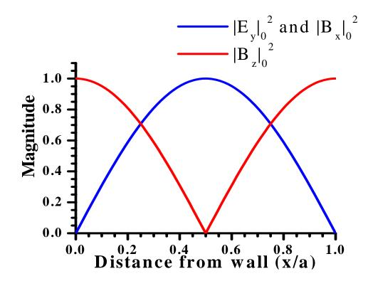
Figure A.1: A plot of the field structure of the TE<sub>10</sub> mode of a waveguide in the transverse plane. Each field is normalized to its maximum value. The blue curve shows  $|E_y|_0^2$  and  $|B_x|_0^2$ , and the red curve shows  $|B_z|_0^2$ .
