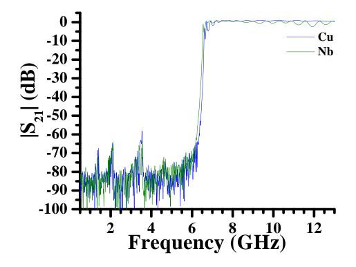
Figure 4.3: A plot of the electromagnetic transmission,  $|S_{21}|$ , versus frequency for an empty Ag-plated brass X-band waveguide, shown as a blue curve, and an empty Nb X-band waveguide, shown as a green curve. The data were taken at room temperature.
