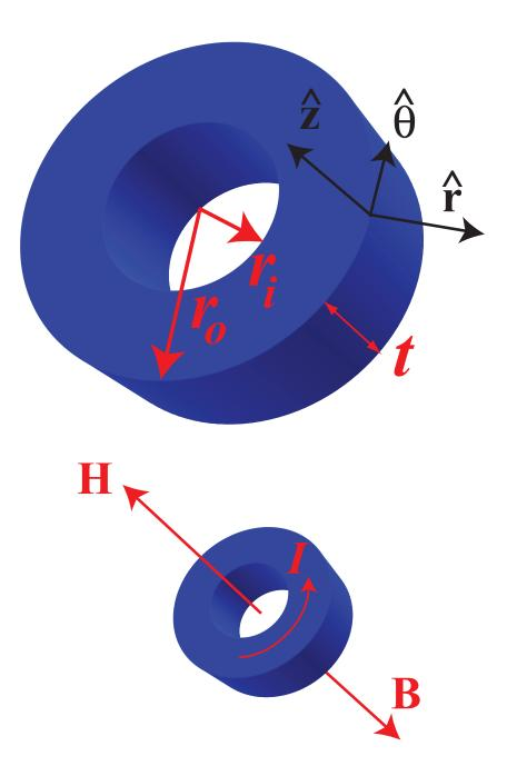
Figure 2.11: Top: A closed ring with inner radius  $r_i$ , outer radius  $r_o$ , and thickness t. The black axes show the cylindrical coordinate axes. Bottom: A closed ring with an applied magnetic field, **B**, inducing a current, I, that generates an H field, **H**.
