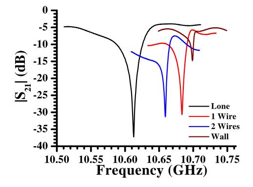
Figure 5.24: A plot of the electromagnetic transmission,  $|S_{21}|$ , versus frequency for the single Nb split-ring resonator- $\beta$  in an otherwise empty Nb X-band waveguide, with various perturbations. All Nb split-ring resonator orientations were plane-parallel gap-orthogonal.
