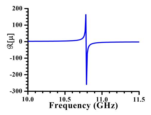
Figure 5.8: A plot of the real part of the permeability,  $\Re[\mu]$ , versus frequency, for Equation (2.97), using the fit parameter values in Table (5.1).
