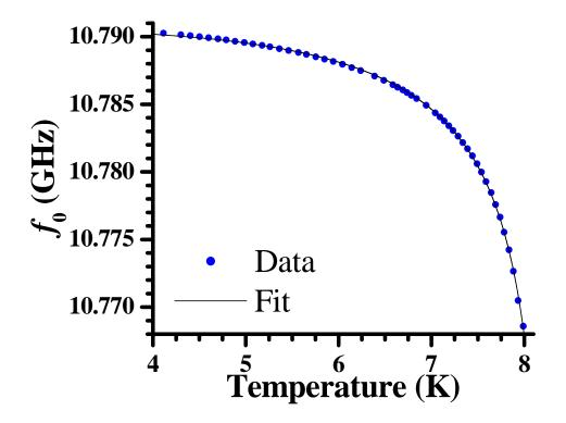
Figure 5.10: A plot of the resonant frequency,  $f_0$ , defined earlier in Figure (5.9), versus temperature for the single Nb split-ring resonator— $\alpha$ . Note that this data is not taken from the data in Figure (5.9), but rather taken at a later time. The blue dots are the data, while the black curve is a fit using Equation (2.151).
