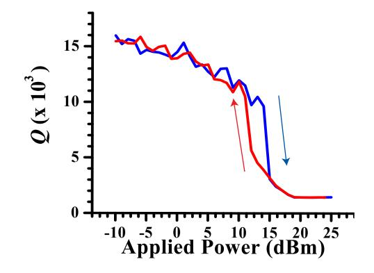
Figure 5.17: A plot of the quality factor, Q, versus applied power for the single Nb split-ring resonator- $\beta$  in the Ag-plated brass X-band waveguide, immersed in liquid Helium. The blue curve is increasing power, and the red curve is decreasing power.
