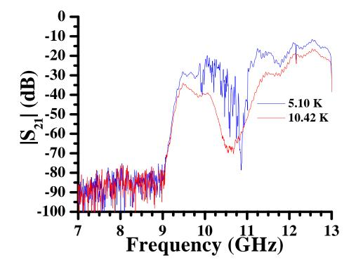
Figure 6.4: A plot of the electromagnetic transmission,  $|S_{21}|$ , versus frequency for an array of 216 Nb split-ring resonators in a Nb wire array measuring five wires transversely and eighteen wires longitudinally, with a lattice parameter of a = 7.19 mm. The blue curve was measured at 5.10 K and the green curve was measured at 10.42 K. The distance separating the wires and Nb split-ring resonator was approximately d = 2.54 mm.
