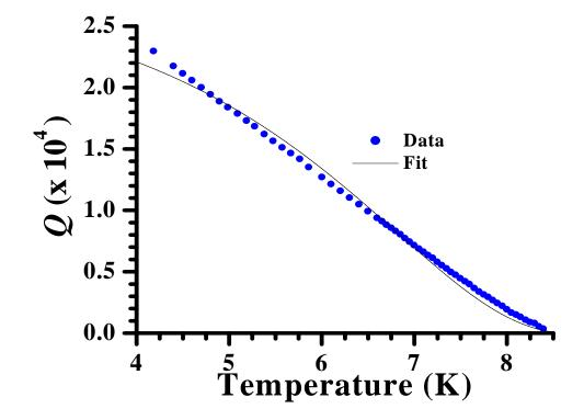
Figure 6.10: A plot of the quality factor, Q, versus temperature for the single Nb split-ring resonator— $\alpha$  in a Nb wire array measuring five rows transversely and seven rows longitudinally, as in Figure (6.8), inside the Nb X-band waveguide. The blue dots are the data, while the black curve is a fit using Equation (2.161).
