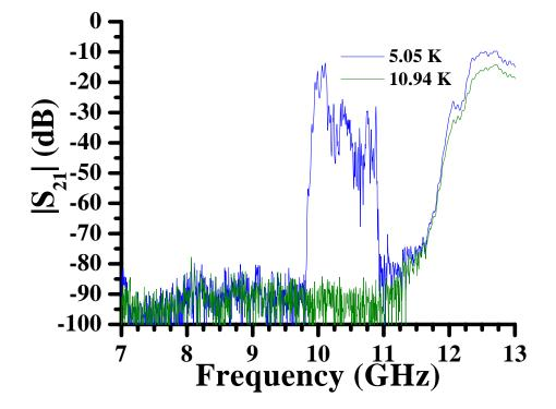
Figure 6.1: A plot of the electromagnetic transmission,  $|S_{21}|$ , versus frequency for an array of 216 Nb split-ring resonators in a Nb wire array measuring five wires transversely and eighteen wires longitudinally, with a lattice parameter of a = 5.08 mm. The blue curve was measured at 5.05 K and the green curve was measured at 10.94 K. The distance separating the wires and Nb split-ring resonator was approximately d = 2.54 mm.
