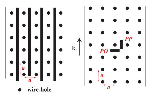
Figure 3.10: A metallic wire array, shown as black circles with lattice parameter, a, and an array of split-ring resonators, shown as the black rectangles. The view is along the y-axis in Figure (2.3). Left: Long arrays of split-ring resonators and wires. Right: A single split-ring resonator in the wire array. The positions are labeled PP for plane-parallel, and PO for plane-orthogonal. The orientation is in reference to the wave vector, shown in the middle of the figure.
