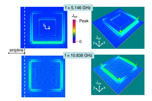
Figure 5.18: A plot of the photoresponse of a YBa<sub>2</sub>Cu<sub>3</sub>O<sub>7- $\delta$ </sub> split-ring resonator. (*a*): Outer ring resonance at 5.146 GHz; (*b*): Outer ring resonance at 10.838 GHz. (*c*) and (*d*): Three dimensional plots of (*a*) and (*b*), respectively.
