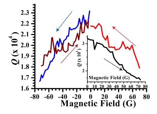
Figure 5.13: A plot of the quality factor, Q, versus an applied dc H field for the single Nb split-ring resonator- $\beta$  in an otherwise empty Agplated brass X-band waveguide, immersed in liquid Helium. The arrows indicate the direction of the change of the applied dc H field.
