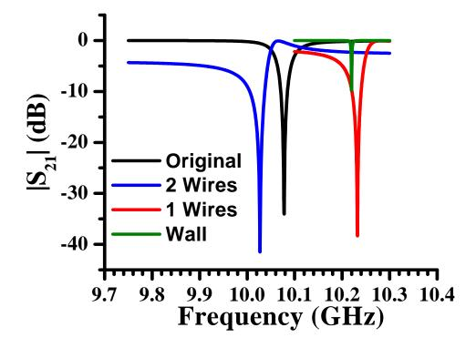
Figure 5.25: A plot of the electromagnetic transmission,  $|S_{21}|$ , versus frequency for a simulation of a single perfect electric conductor splitring resonator in an otherwise empty X-band waveguide, with various perturbations.
